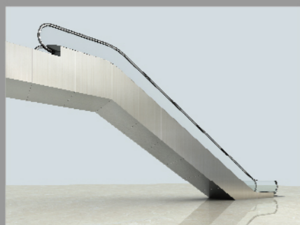
Plan 2-1 Glass interior plate, External decoration plate perpendicular to horizontal plane without lighting.
